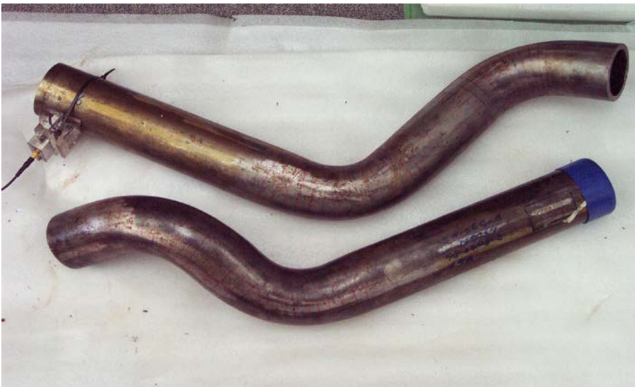
Figure 2: Sample pipes used in prototype development. One sample has an axial EDM notch in the middle of a bend the other sample is free of cracking.
